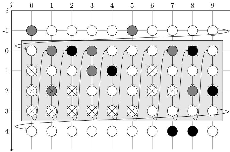
Figure 4: Significant propagation pass on the bit-plane  $n = 4$ .
