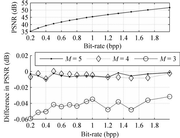
Fig. 7. Rate-distortion curve with JPEG2000 and difference of PSNR with combined contexts.
