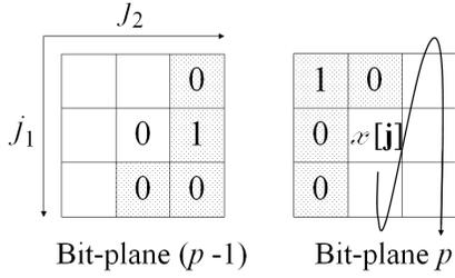
**Fig. 1.** Example of a modeling context  $C$  for the ZC primitive. Here the 0 and 1 denote the coefficient significance. As the scan follows the arrow, this modeling context is composed of the significance of four coefficients in the bit-plane  $(p - 1)$  and the significance state of the four other neighbors in the bit-plane  $p$ . In this particular case  $\mathbf{m} = (0\ 0\ 1\ 0\ 1\ 0\ 0\ 0)$  and  $m = 6$ .
